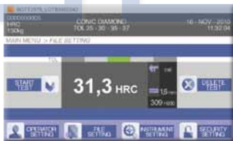
At the end of the test, hardness result, unit of measure and tolerance range are displayed. Further information, such as minimum measurable thickness or the presence of a calibration, can be viewed if the proper function has been previously activated.
