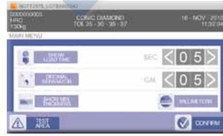
This menu enables setting the parameters of the hardness test such as Load Time, Minimum Thickness, Calibration adjustment.
