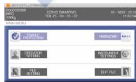
This menu enables setting a password to protect some functions, which Operator Setting, File Setting, Instrument Setting, Edit File.
