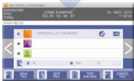
This menu enables creating and editing the different operation environments, which are called files. After entering, the list of existing files is displayed.
