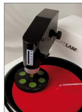
With the SPRINGLAM ® head use the SMARTLAM ® as a semi-automatic polisher.
