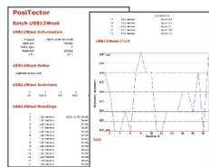
A simple gage interface to retrieve data in a manner similar to USB flash drives or cameras. No software to install or internet connection required. Measurement data can be printed quickly from a formatted HTML report or exported in .csv format for further analysis in spreadsheets.
